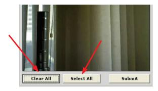
To configure a particular area for motion detection, simply click and hold down the mouse left button and move diagonally to select a desired area. You can do it repetitively to configure multiple areas for motion detection:
