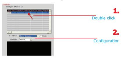
Finally, select the desired intelligent detection function from the "Event Mode" drop-down and make sure "Enable" is ticked:
