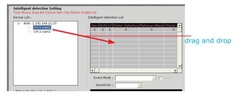
Double click on the desired channel in the "Intelligent Detection List" to enable configuration:
