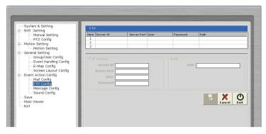
You can configure up to three FTP servers in which you can select later and use them for different event trigger conditions.
