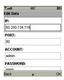
To log into the DVR, you need to enter the logging-in DVR information. Find "Add" under the "Menu" then enter logging-in DVR's IP address, Port number, account name and password. Press "Add" to save this information after entering.
