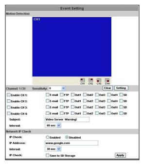
VIDEO SERVER supports one motion detection area on each channel. When the motion is triggered, it can send out the video to a certain email address or upload the video to FTP. If the user has a SD Card, they can
