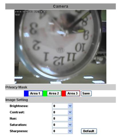
For the security purpose, there are three areas can be setup for privacy mask. Click Area button first and pull a area on the above image. Finally, click Save button to reserve the setting.
