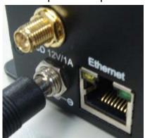
ii. Connect Video Server to PC or network with Ethernet cable
