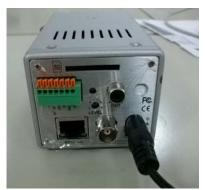
ii. Connect IP Cam to PC or network with Ethernet cable
