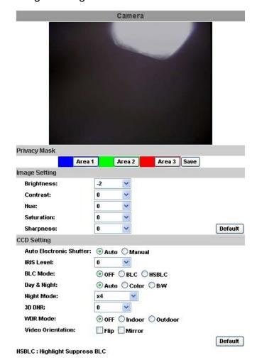
For the security purpose, there are three areas can be setup for privacy mask. Click Area button first and pull a area on the above image. Finally, click Save button to reserve the setting.
