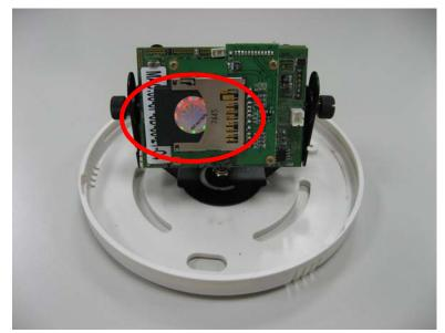
Please Insert SD card before use it. Make sure pushing SD card into the slot completely.
