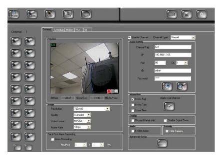
b. There are 18 channels listed on the left side of the administrator page. Users can use to switch 1-18, 19-36 channels. Moreover, users can use either keyboard to enter the setup values,
