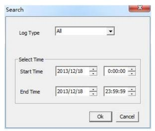
Click the "system configuration" on the menu bar, open "Journal Manage" window and click the Equipment Journal, below it click search, then the pop-up dialog box shown in the diagram below: Chose the journal type (All/The motion detecting alarm/IO input alarm), Equipment, The date time; Click Ok, then query log success.
