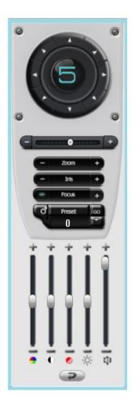
Equipment can achieve to PTZ control function through RS485 external connect with PTZ device, also control the run speed of PTZ ,test the Zoom , adjust focus and Iris , c preset , and brightness contrast etc.
