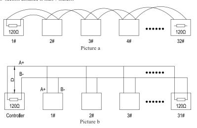
Picture b is RS485 bus cable  $120\Omega$  terminal resistance jumper. To avoid 485 signal reflex, connect  $120\Omega$  terminal resistance at the end the 485 bus cable. The middle equipments must disconnect terminal resistance.
