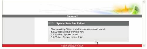
• **STEP2**: The Action LED indicator will light down to indicate that the IP device is rebooting. After around 30 seconds, the Action LED will light up again to indicate that the reboot is completed.
