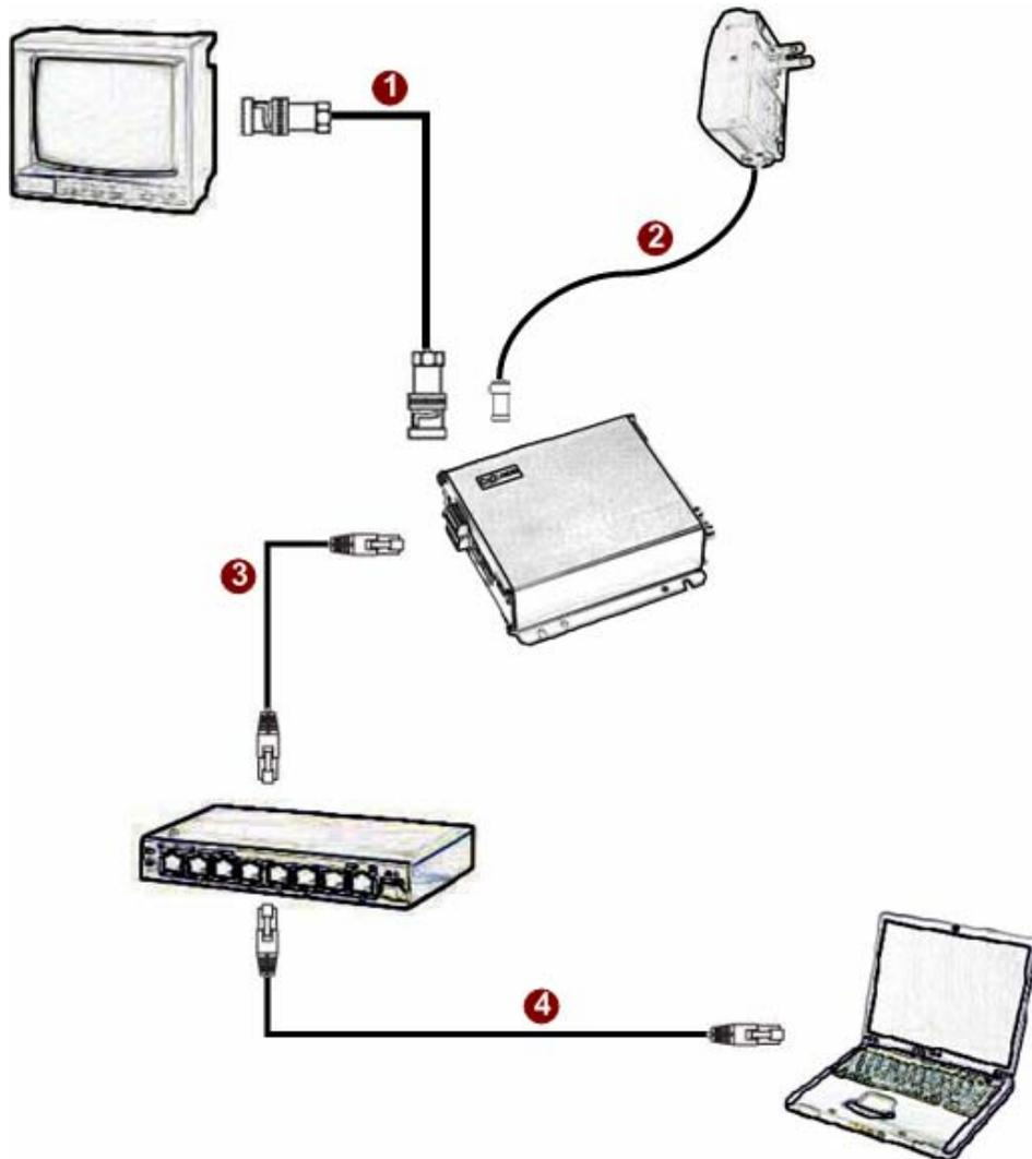
1. Connect an analog monitor to video server video out (BNC connector).
