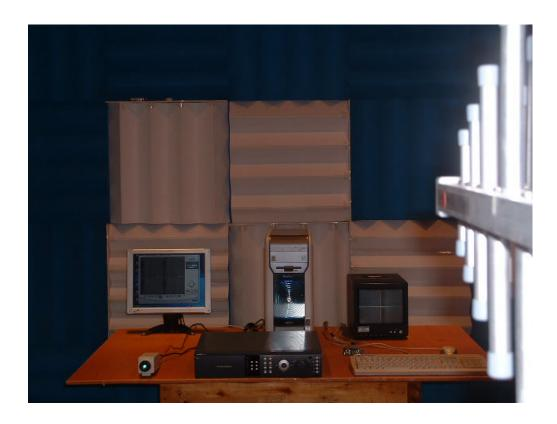
Radiated radio-frequency electromagnetic field
