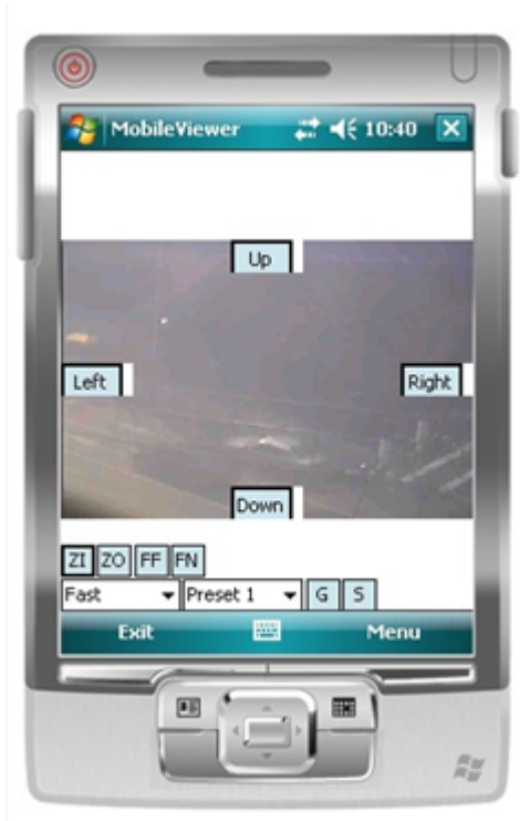
Figure 4.86. PTZF control screen
